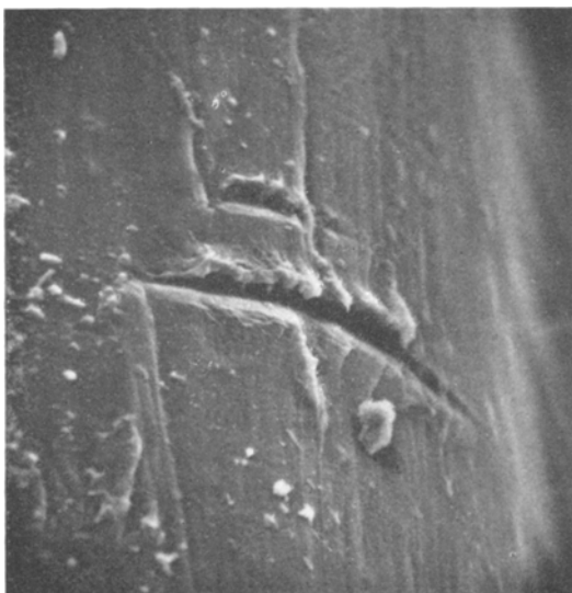
Figure 6 Points of fracture initiation in nylon 66 mono-filament (a \times 3600 ; b \times 4650 ).
